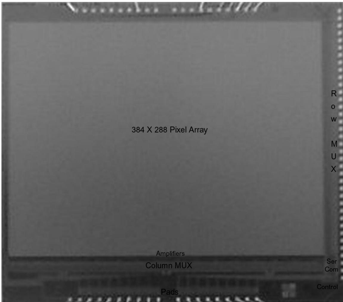
Fig. 6. Photograph of the readout chip. The die size is 10.46 mm x 9.24 mm. 109
